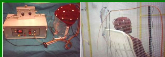
Fig. 1.- TMS stimulator, mod. MG28TR10 (left). Subject sitting inside the Faraday chamber. Recording cap and amplifier are also shown here, (right).
